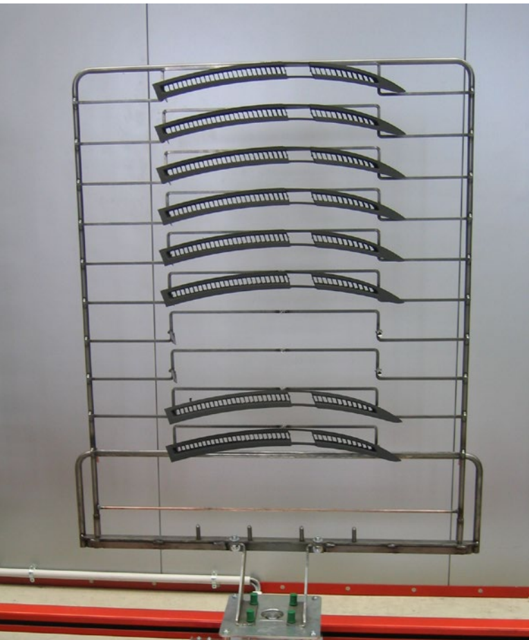
Metal matrix rack for a floor conveyor. The plastic grid is held in place by wire brackets and two clamping springs.
