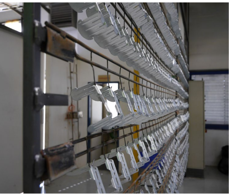
Hook shaft vertical for universal holding of different sheet metal parts.
