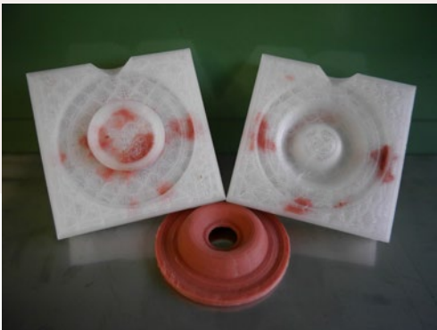
Two 3D-printed mould halves with hand-cast silicone moulded part.
