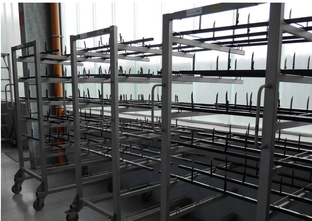
Storage and drying trolley for painting skewers.
