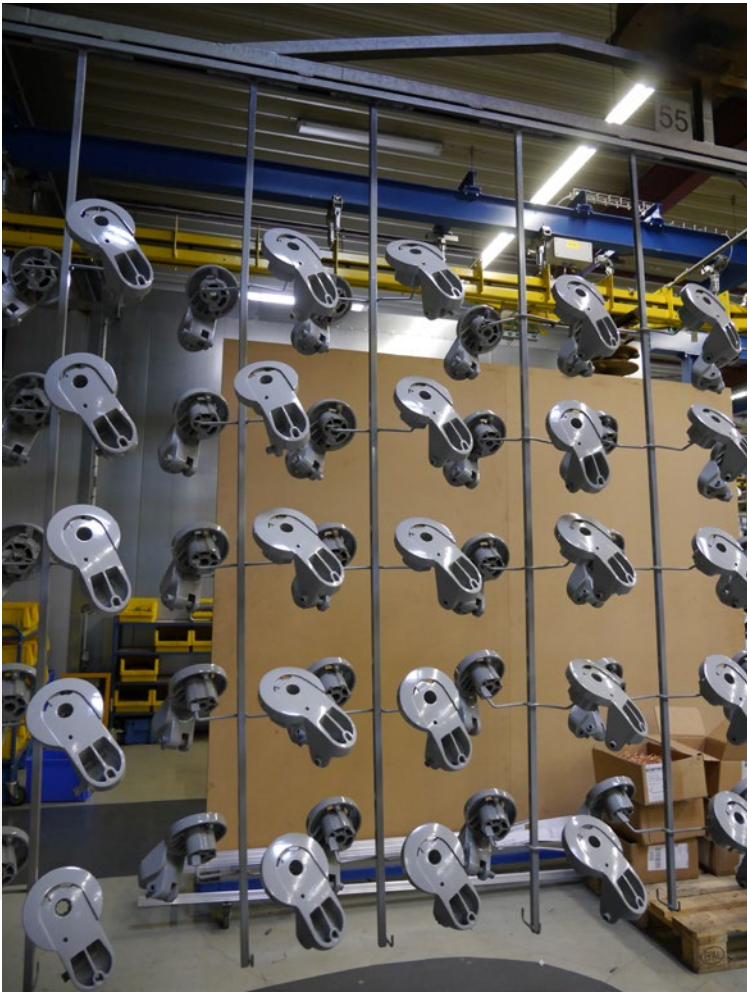
Vertical hanger with firmly welded support arms. The components are offset on both sides.
