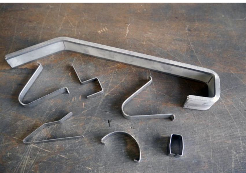
Spring clips made of VA spring steel and suspension hooks made of flat material (30 x 8 mm).
