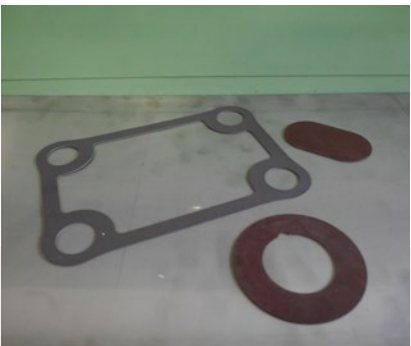
Contour cuts made of magnetic silicone rubber
