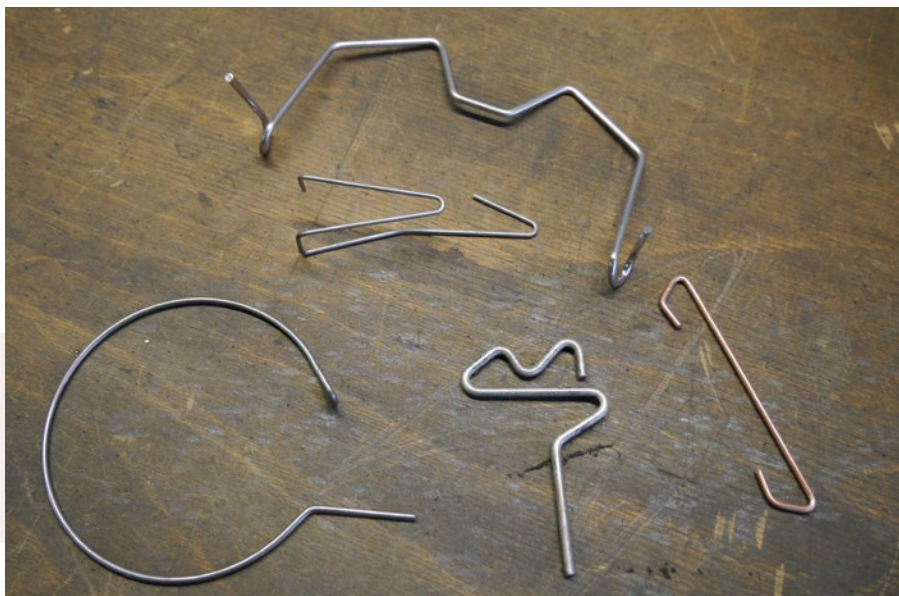
Two-dimensional and three-dimensional wire bending parts with diameters between 1.5 and 3 mm.
