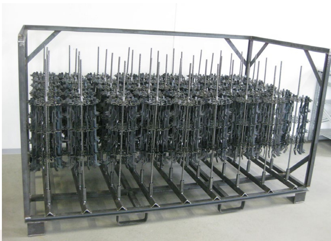
Transport and storage box for painting fixtures with optimum use of space.
