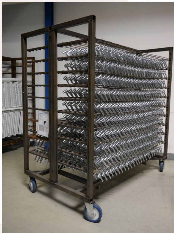
Transport and storage trolley for painting crossbars.
