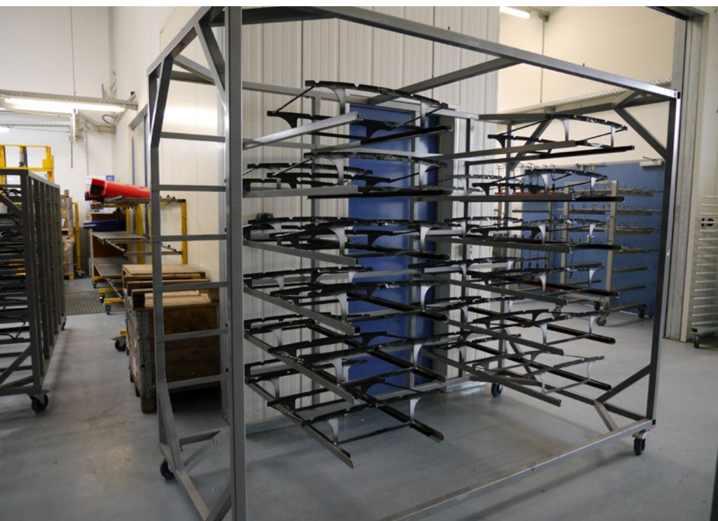
Storage and drying trolley for painting racks.
